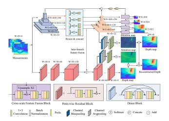
Figure 2. Dual-branch depth reconstruction network.
